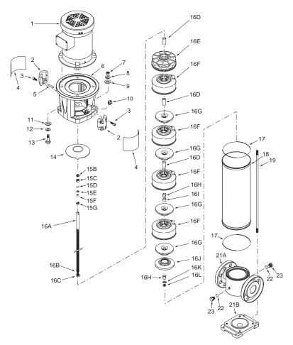
Figure 17. Exploded View of PVMX8 and PVMX16.
