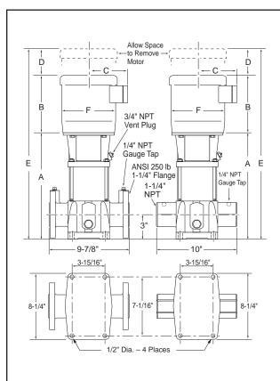
Figure 2A. Height, width and baseplate dimensions for PVM2 and PVM4 Series pumps.
