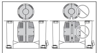
Figure 10A. Make sure that the coupling halves are evenly tightened.
