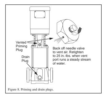
1. Close the discharge isolating valve and loosen the needle valve located in the assembly in the pump head (Figure 8). Do not remove the needle valve.
