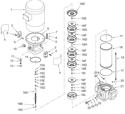
Figure 14. Exploded View of PVM2 and PVM4.
