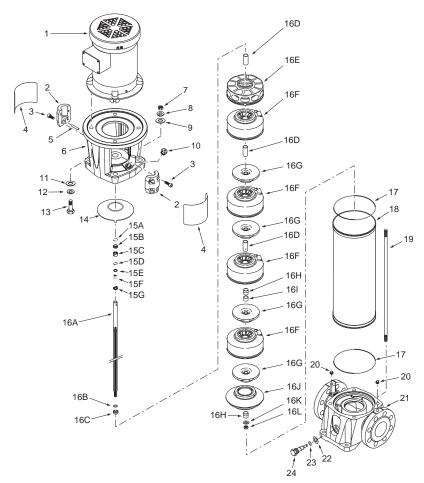
Figure 15. Exploded View of PVM8 and PVM16.
