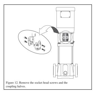
TWO PART MECHANICAL SEAL/DISASSEMBLY. See Table VII to determine which seal your model has.
