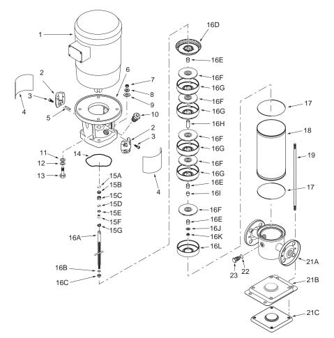
Figure 16. Exploded View of PVMX2 and PVMX4.
