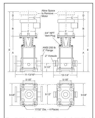
Figure 3B. Height, width, and baseplate dimensions for PVMX8 and PVMX16 Series pumps.
